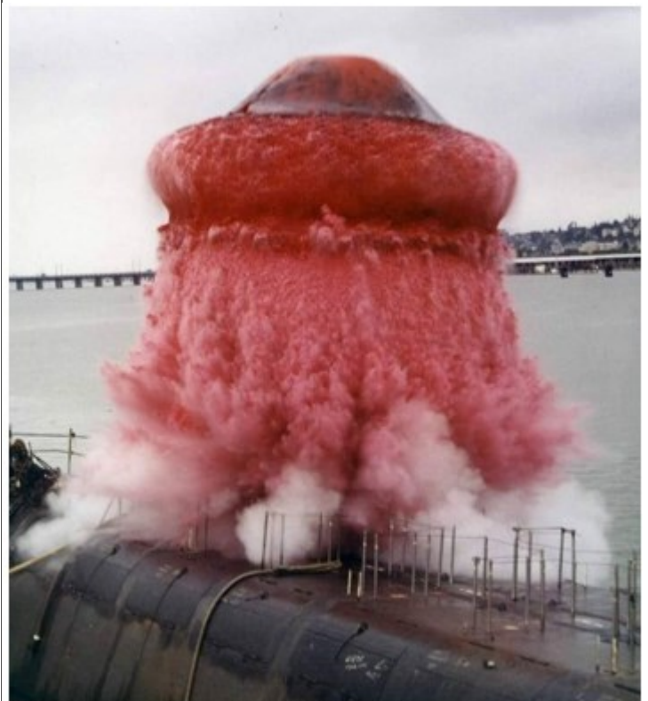
USS Daniel Boone (SSBN-629) firing a colored water slug, at Mare Island in February 1964
